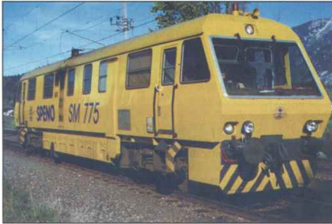
Fig. 2: Speno SM 775 Rail Surface Recording Vehicle
