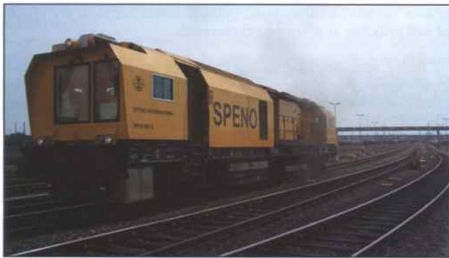
Fig. 7: Speno RR 16 MS-2 Turnout Grinding Machine
